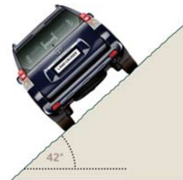
Limit angle of vehicle turnover
