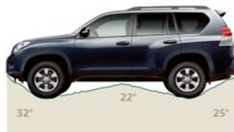
Approach, ramp break over and departure angles
